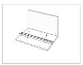
**U-Shape Extrusion:** Ideal for facades with straight lines, suitable for vertical or horizontal light emission.
